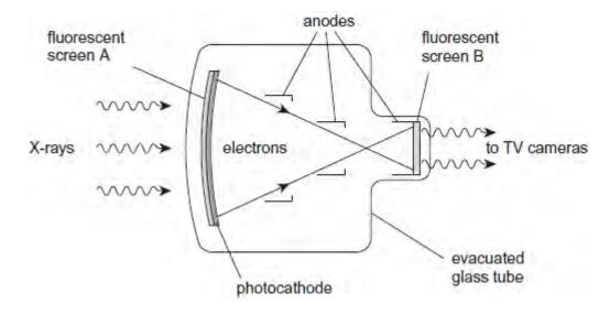
State the purpose of each of the following components of the intensifier.
